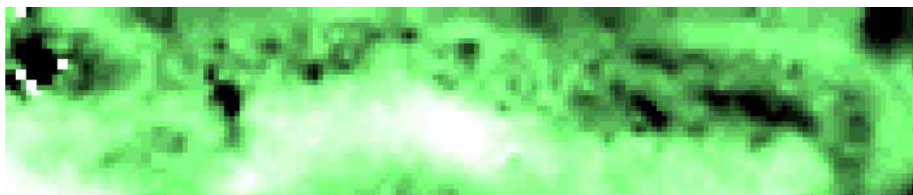
Processed plot of earth resistance survey. Light areas represent low resistance, dark areas high resistance. (The plot is 90m long, with North to the right)
