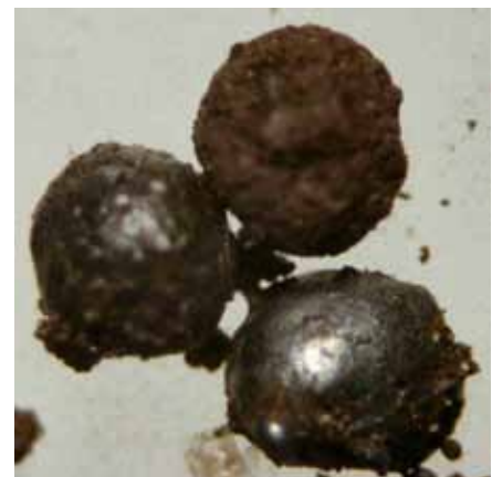
Metallic droplets. The largest is c. 1mm diameter
